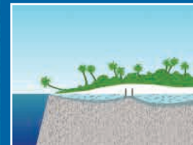
3. A well taking more water than diagram 2 results in brackish and saline groundwater entering the well. This most commonly occurs with stop-start electric suction pumps.
