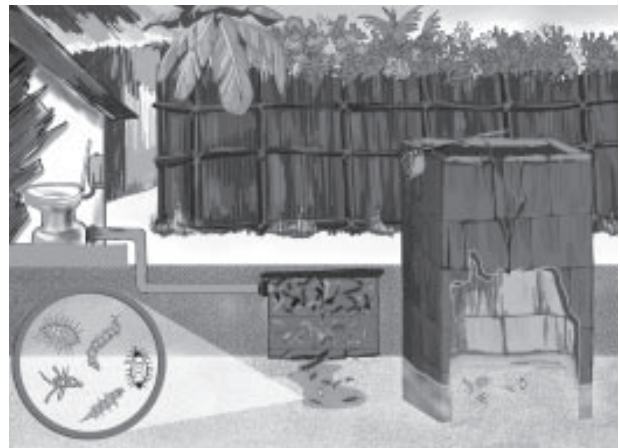
Leaking septic tanks commonly contaminate well water in the Maldives.
