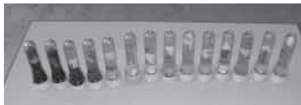
Water samples tested using H 2 S paper strip test.
